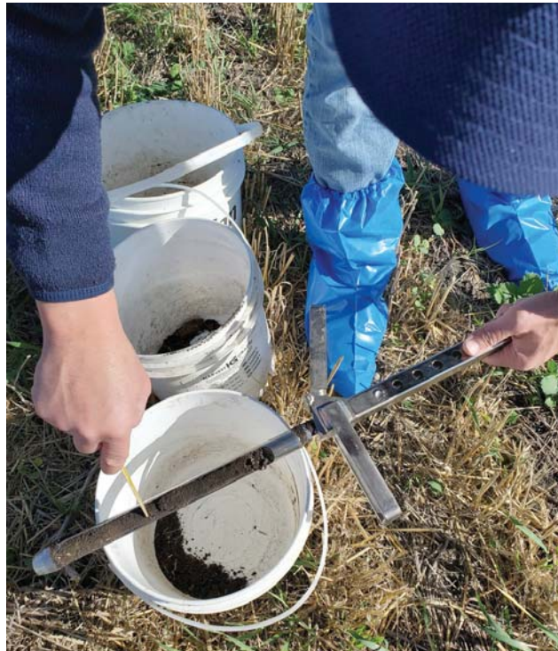
When soil sampling, divide each core into two or three soil depths and put them into separate pails. Submit separate composite blends for each depth.
