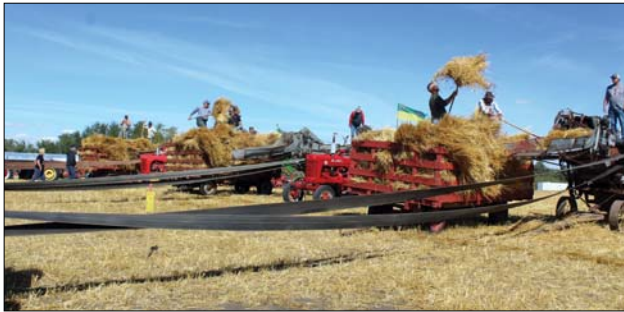
Three vintage threshing machines at work, which are powered by the long canvas pullet belts and tractor power.
