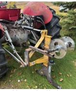
A homemade cable plow to pull the wire
